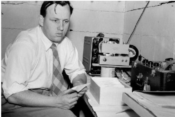
A cathode-ray oscilloscope was used to take measurements from the waveform of their recordings.
