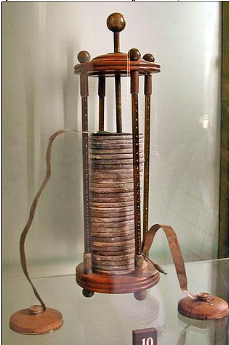
Figure 3. A battery (or voltaic pile) first built by Alessandro Volta. He used discs of zinc and silver, separated by cardboard soaked in brine. ( http://en.Wikipedia.org/wiki/Alessandro_Volta )
